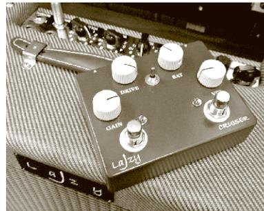
You have three gain stages – an input and an output stage, and between those two you generate the boost. You set the Gain at the first stage with the control. That goes to the output gain
