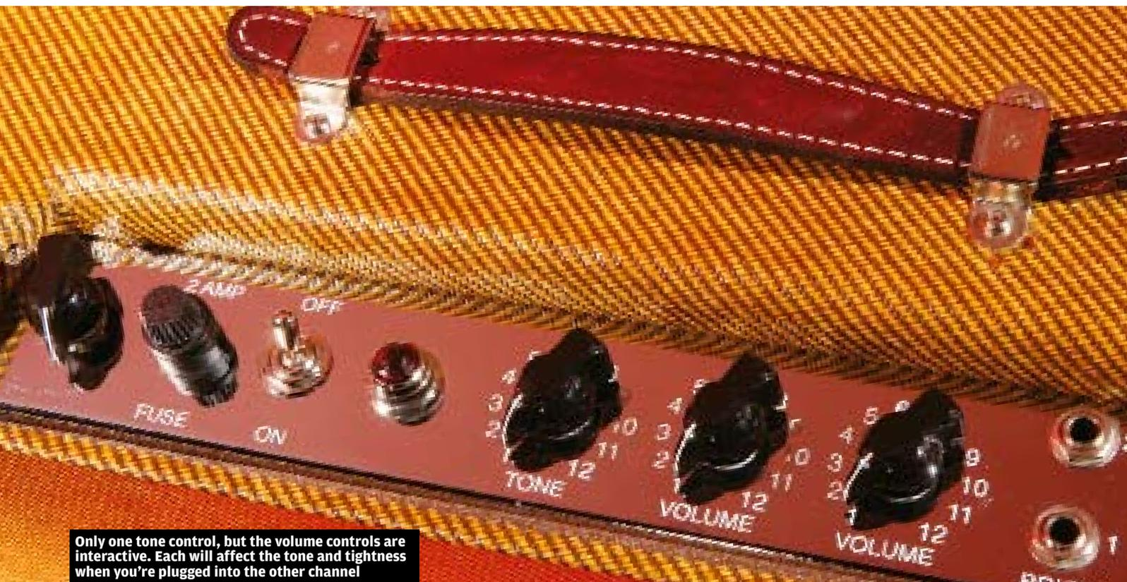
Only one tone control, but the volume controls are interactive. Each will affect the tone and tightness when you're plugged into the other channel
