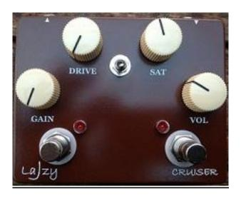
**DRIVE** --- controls drive circuit input **SAT** --- controls drive circuit output
