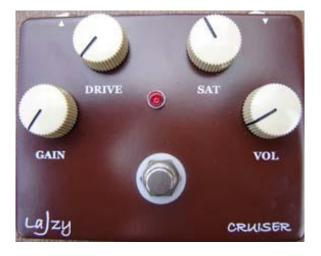
GAIN --- controls Input Gain DRIVE --- controls Drive level SAT --- controls 3 modes of clipping /comp VOL --- controls Output Level
